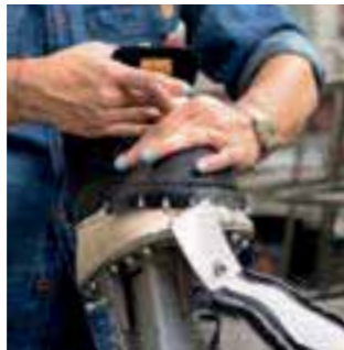
5 INSERIMENTO MEMBRANA WATER SHIELD Water Shield membrane insertion / Einsetzen Water Shield Mem- bran
